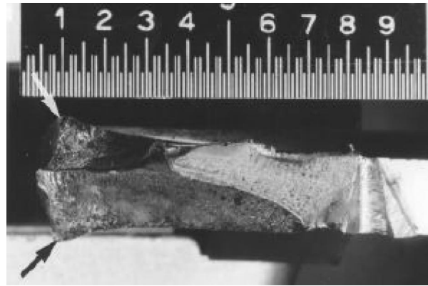
Fig. 3 Plan view of opened crack segment. Arrows locate two origins at the bottom corners on opposite sides of the airfoil. (Scale divisions=0.01 in.)
