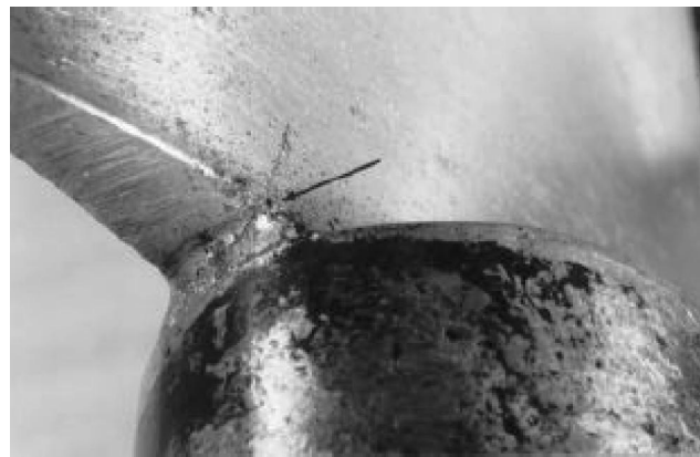
Fig. 4 Large corrosion pit (arrow) at IGV crack origin
