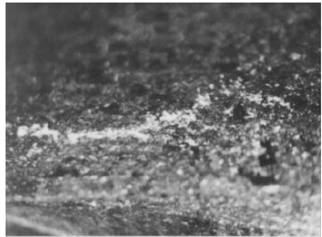
Fig. 8 Metallic wear particles (bright) on bushing contact surface (original 20X)
